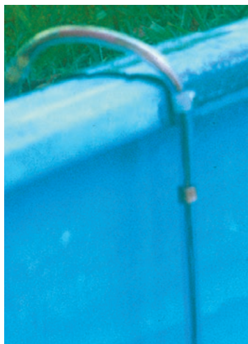
The top of the water level sensor can be secured to the tank using a suitable bracket.
